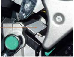
The strategic integrated RFID design increases encoding accuracies by reducing the electro-mechanical interferences within the printer. This ensures maximum precision labels and RFID tags.
