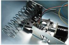
Heavy Duty Latch Mechanism
