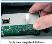
USB, LAN, Serial, Parallel, WLAN, CloudPRNT, AirPrint, and WebPRNT\*
