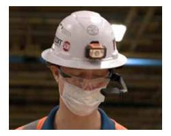
A single onsite Honeywell employee wearing a RealWear device is able to share what they are seeing and engage with offsite expert colleagues through Microsoft Teams in real time. The voice-activated controls enable the wearer to use the various functions — including viewing documents on the highresolution micro-display, contacting coworkers on Teams, and more — without taking their hands or attention off of complicated machinery or equipment.
