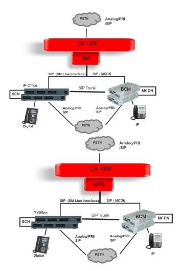
This configuration allows migration for a network of BCM and CS1000 to the IP Office step by step by adding IP Office systems to it.
