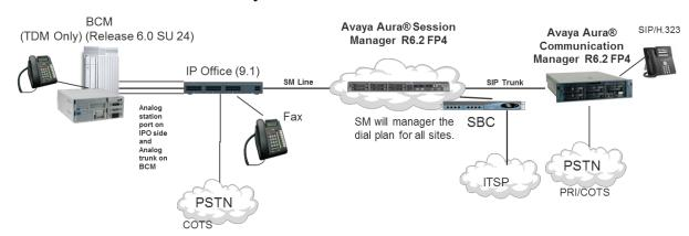
IP Office R11.0 supports a deployment scenario for IP Office, where IP Office acts as a SIP Gateway for a Nortel BCM and/or a Norstar telephony system. The following use cases are supported:
