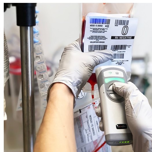
Programming the top-mounted buttons enables CR2700 to perform two distinct functions, such as Rx scanning and sample tracking.
