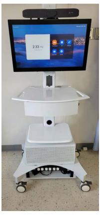
With its small footprint and well-designed features, the TMP-200 was the ideal choice for ARH. The solution includes the Poly Studio X50 accessing Zoom wirelessly. The slide-out draw provides easy access to stethoscopes and other devices required for a patient exam and diagnosis. The backup battery provides the needed power for hours of exams. In addition, the TMP-200 also provides a sustainable and reliable backbone for future growth and use case.
