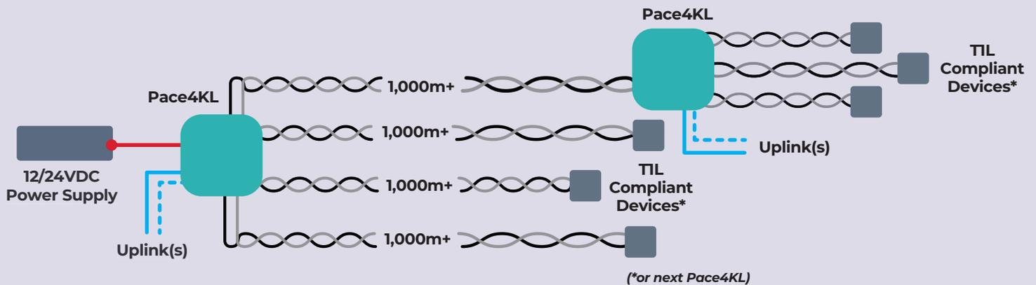
The Pace4KL T1L adaptor/switch can connect directly to up to four 3cg, T1L devices and feature dual network uplink ports. An additional Pace4KL can be added to the remote end to connect more compliant devices. Network managed versions allow for control, monitoring, and reporting of power diagnostics and feature a single network uplink port.
