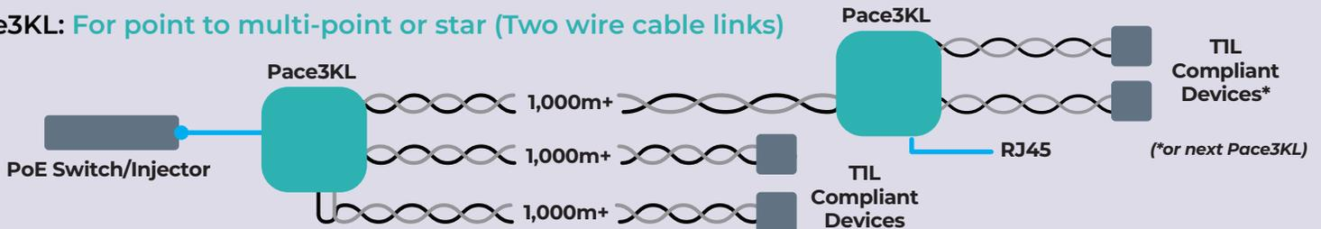
The above scheme shows the first Pace3KL in a typical star configuration, while the second Pace3KL shows how to configure for a continued multi-point drop-off using additional T1L switch to connect T1L compliant devices in multiple locations.
