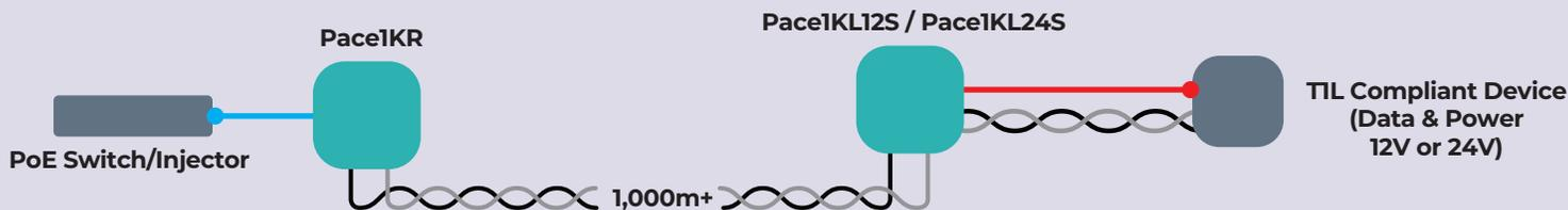
The above setup allows standard TIL data to communicate directly with the TIL remote device, but also splits out 24VDC (Pace1KL12S for 12VDC) to power the same device, thus saving a remote power supply. Since 802.3cg SCCL SPoE/PoDL capable devices are not popular, the above setup facilitates power for any TIL device that is powered by 12V or 24V, as currently are more popular on the market.
