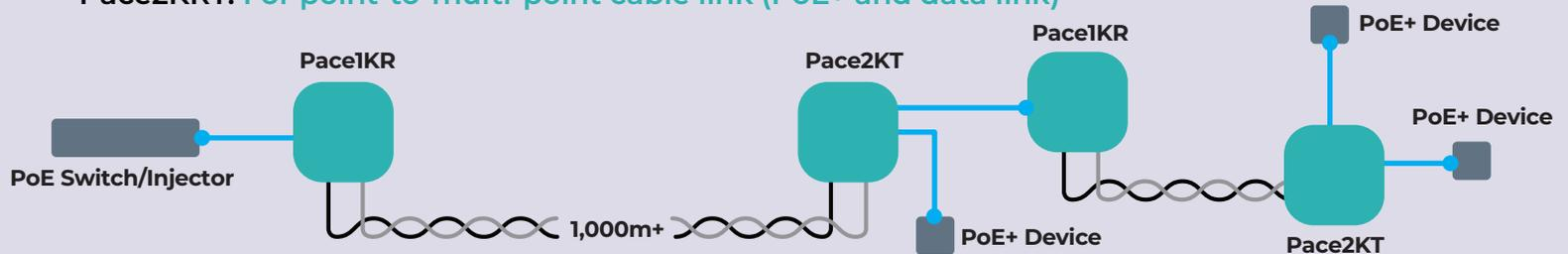
In the above setups the remote end device/s can operate with POE enabled or not. If enabled, remote power supply is not required. POE can also deliver power more efficiently than SPOE Classes 10-12.
