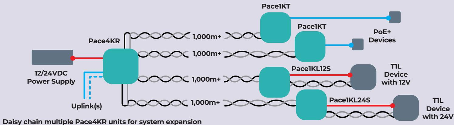
The Pace4KR adaptor/switch feature two network uplink ports and can be paired with four Pace1KT adaptors to remote PoE devices. Pace4KR can also be paired with up to four Pace1KL12S or Pace1KL24S TIL media adaptor/splitters to TIL devices and split power. Network managed versions allow for control, monitoring, and reporting of power diagnostics and feature a single network uplink port.
