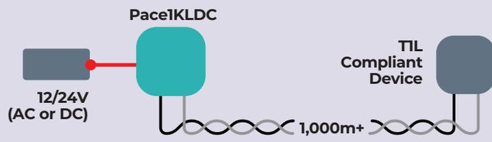
**Pace1KRL12S (12V) | Pace1KRL24S (24V) For point-to-point cable link (TIL Data & Split Power Link):**
