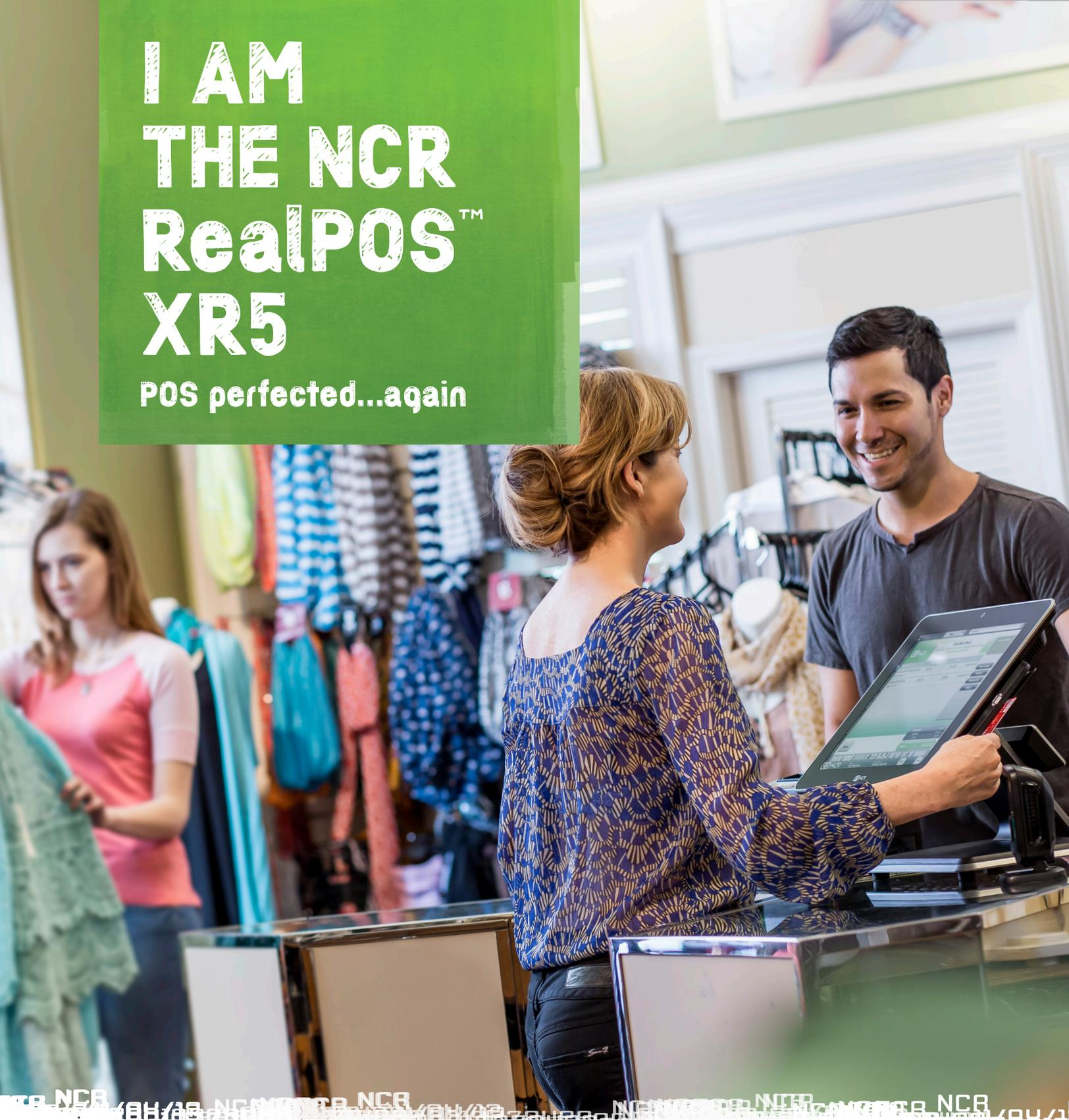
The NCR RealPOS XR5 is an energy efficient, fan-less, multi-touch, point-of-sale (POS) terminal packaged in our stylish X-Series all-in-one design
